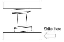
Figure 3-4: Adjusting the Locating Tool
