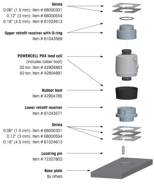
Figure 2-4: Assembly for Receiver Variant 2 "Retrofit"
