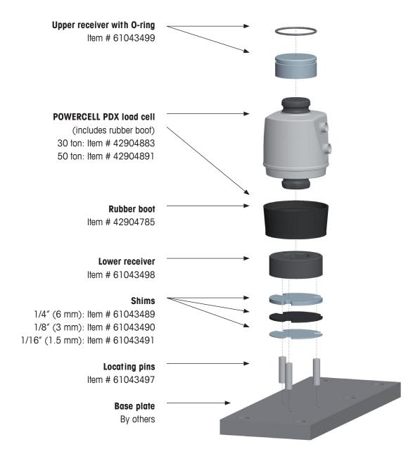
Figure 2-2: Assembly for Receiver Variant 1 "Standard"
