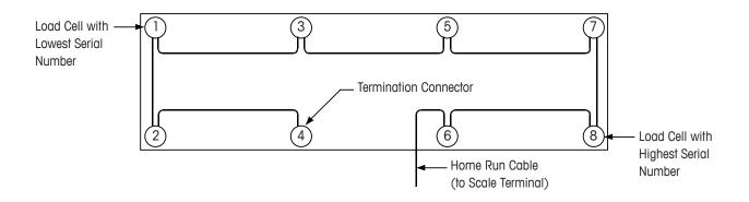
Figure 3-5: Cable Routing for POWERCELL PDX Load Cell Network
