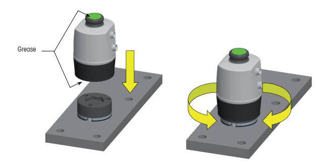
Figure 3-6: Installing the Load Cell
