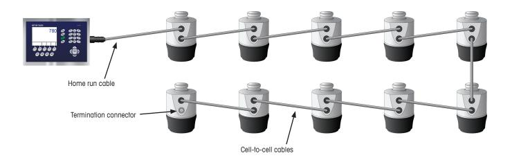
Figure 2-6: POWERCELL PDX Load Cell Network
