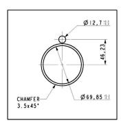
Figure 2-5: Dimensions for Receiver Variant 2 "Retrofit"
