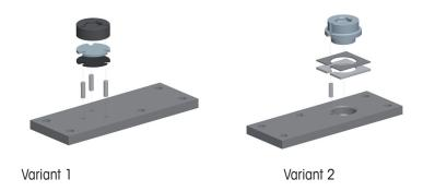
Figure 3-1: Locating Pin Installation
